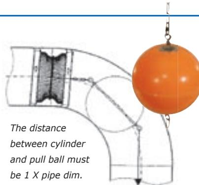
*The distance between cylinder and pull ball must be 1 X pipe dim.*
